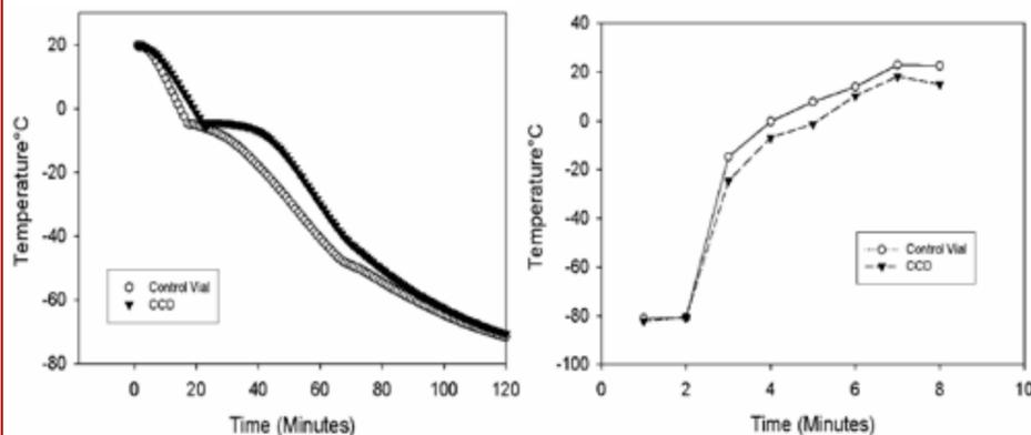
**Figure 3:** A: Temperature-Time history experienced by the cells in CCD and Corning™ cryo-vials when 10%DMSO was used as CPA. B: The post-thaw viability of DPSCs in CCD and control vials (Corning™ vials) when cryopreserved with 10%DMSO and Cryostor™ (CS-10) as CPAs
