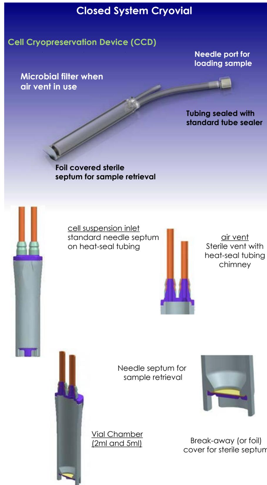
**Figure 1:** Concept of Cell Cryopreservation Device (CCD)
